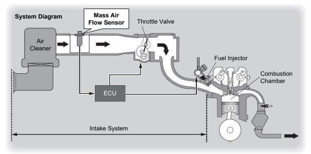
The two following mounting types are available for the mass air flow sensor:
