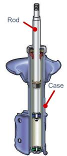
of rolling, which can cause anxiety in drivers. When the performance of the shock absorber has degraded after prolonged use, drivers would frequently become uncomfortable owing to such rolling impression. In this case, a level of ride comfort and vehicle operability similar to those of a new car can be obtained by replacing the shock absorbers with new ones. The shock absorbers are important components that provide vehicle safety and ride comfort.
